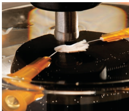
A high-frequency ultrasound probe from Dr. Shung’s lab, used to scan small tissue samples, is aiding studies at The Saban Research Institute of the heart-regenerative qualities of zebrafish.
